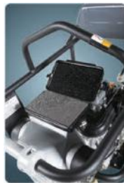
Double air filter is available for H12-2D,Gx100 engine
